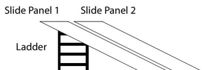
**CONFIGURATION** • One ladder, two equal slide panels—side by side (in *parallel*).
