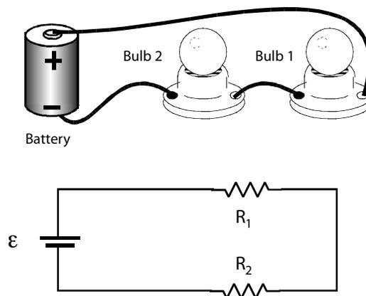
**CONFIGURATION** • One battery, two equal light bulbs—one after the other (in *series*).
