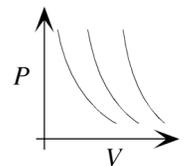
A **Carnot engine** operates along two adiabats and two isotherms. Heat is added along the high isotherm and ejected along the low isotherm. Volume increases and pressure drops along the high isotherm and adiabat; volume decreases and pressure increases along the low isotherm and adiabat. Negative work is done on the gas during expansion; positive work is done on the gas during compression.
