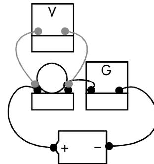
2. Consider a pair of uncharged parallel plates. A voltmeter is attached across the plates and a galvanometer is connected to one plate. A bulb is connected in series with the galvanometer and a battery is added to complete the circuit.
