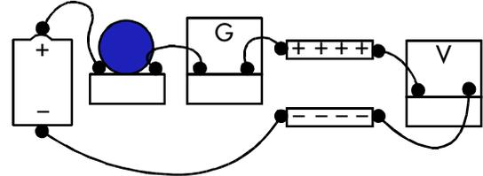
3. At this point, one plate has a considerable positive charge and the other has a considerable negative charge, Next, the battery is removed. At this point, the bulb is unlit, there is no current through the wire, but there is a potential across the plates. Next, the wires leading to it are connected to each other. This creates a path from the positive plate to the negative plate. Of course, for charge to move from one plate to the other, it must pass through the bulb.
